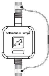
Figure 6: Earth continuity (4mm 2 earth connection cable)
