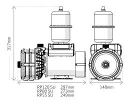
All Right Pumps have the standard inlet/outlet configuration for ease of replacement.
