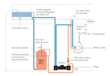
CT or Right pump range twin ended positive head with up and over pipework and natural flow of 1Litre/min per side.
