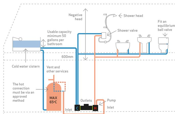
CT pump range twin ended universal to a bathroom in a loft conversion.
