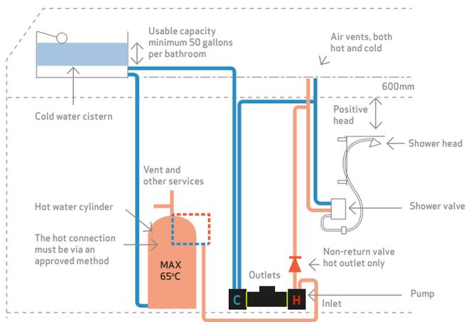
CT pump range twin ended positive head with up and over pipework and natural flow of 1 Litre/min per side.
