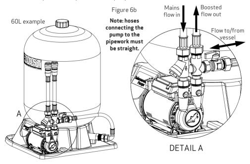
Isolators on anti-vibration hoses (pumped units only)
