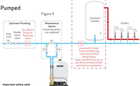
The maximum theoretical pressure after the AccuBoost is the setting of the AccuBoost pressure reducing valve plus the output of the pump (3 bar). The total of these must not exceed the setting of the unvented cylinder pressure reducing valve/safety valve. The setting of the AccuBoost pressure reducing valve may need to be adjusted down to suit.
