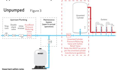
The setting of the AccuBoost pressure reducing valve must be set lower than the setting of the unvented cylinder pressure reducing valve/safety valve and so that the maximum system pressure of the AccuBoost unit is not exceeded. The setting of the AccuBoost pressure reducing valve may need to be adjusted down to suit.
