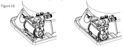
5. Connect the straight end of the vessel hose to the vessel port on the pump and connect the angled end of the vessel hose to the brass vessel connector.
