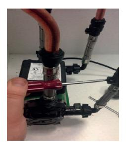
Both sets of hoses can now be removed from the pump - there will be some residual water in the hoses and pump, so it may be worth using a cloth to catch the excess.
