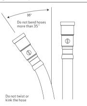
Ideally the AV couplers should be straight, but they must NOT be twisted or bent more than 35° (this invalidates the warranty). See Figure 5 above. Single pumps are designed to boost hot or cold water - supplied with x1 angled, inlet hose and x1 straight, outlet hose
