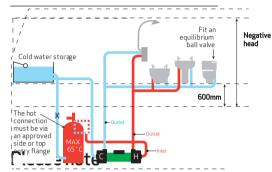
Right universal twin pumps to a whole house system. In these systems TOILETS must be fitted with equilibrium ball valve(s).
