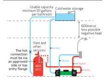
Figure 7: Typical Right Pump Installation - pump located above the cylinder
